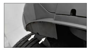
7. Unscrew 2 screws on each side in the bottom part of bumper.
