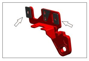
30. When installing the recovery points with RIVAL winch plate, use washers pos. K, in places of fastening with the bolts M16 as shown.
