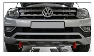
55. Try on the bumper. If necessary, extend the holes for the recovery points, for unobstructed bumper installation.
