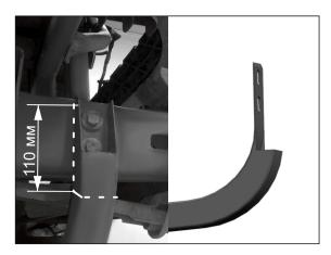
20. To perform step 19, cut the skid plate bracket on the right side, so that it turned out as shown above. To do this, pre-mark the bracket.
