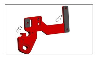
41. When installing the hinge with RIVAL winch plate or OE skid plate, place inserts pos. K and pos. S between the frame and the recovery point. When installing with RIVAL skid plate, use inserts pos. O and pos. T.
