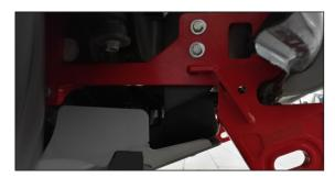
47. Press the recovery point to the frame and high up as possible, tighten all the hardware.
