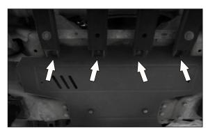
14. Unscrew 4 bolts securing skid plate at the bottom of the car.
