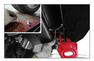
28. Put the insert plate pos. Z, inside the frame through the hole on the inside and pre-bend the wire on the insert plate in place.
