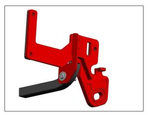
49. Connect the bracket of the OE skid plate with the bracket pos. D using bolt M12x80, washers 12 and nut 12.
