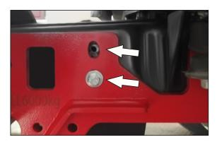
29. Match the holes in the insert plate with the holes in the frame and the recovery point, as shown and tighten bolts M8x40 in them.
