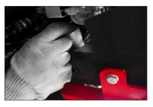
31. Install bushing into the frame at the rear part of the recovery point, on the inside, then screw the bolt M16x100 with washer pos. K, into the body of the recovery poin, on the inside of the frame through the bushing.
