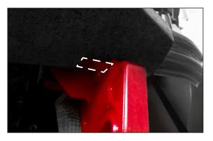
25. Mark the place for cutout on the damper. If recovery points are installed with RIVAL winch plate, perform cutout with 3 mm displacement to lateral sides of the car.
