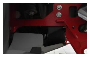
38. Place the recovery point to the car frame by matching the holes, you may screw the bolts M8, mark the place for cutout in the damper (see items 21 and 22).
