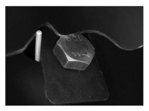
32. Install the bolt M16x120 with washer pos. K, in the hole on the inside of the frame at the front part.
