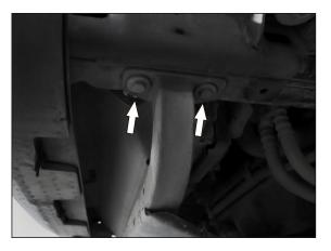
13. Unscrew 2 bolts securing skid plate on the left side.
