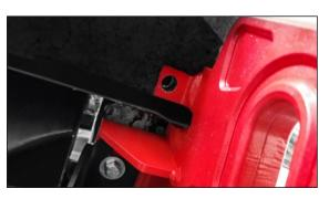
35. Mark the place for drilling across the hole and drill the hole using a drill with diameter of 10.5-11 mm
