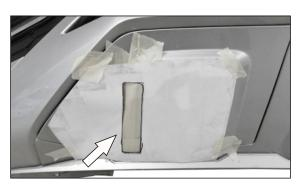
53. Mark the place for cutout in the bumper. Remove the template. Cut a hole in the bumper along the marked path.
