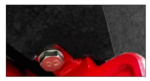
46. Install the bolt M10x35 with washers 10 and the nut M10 into the hole. Place inserts.
