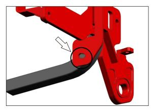
22. Mark the place for drilling and drill a hole with diameter of 12.5-13 mm.
