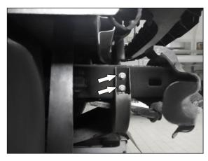
12. Unscrew 2 bolts securing skid plate on the right side.
