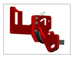
21. Connect together the skid plate, right recovery point and bracket pos. D, using bolts M8.
