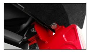
36. Install the bolt M10x35 with washers 10 and the nut M10 into the hole. Place inserts pos. W, if necessary, between the recovery point and the body to eliminate gap.
