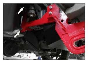
44. Attach the clamp to the recovery point with 2 bolts M12x40. **Do not tighten yet.**
