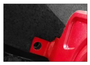
45. Slightly tighten all the hardware, mark and drill the hole with 10.5-11mm drill bit to secure the front bracket (similarly to step 32).
