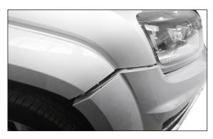
9. Dismantle the bumper. To do this, gently pull the edge of the bumper and unfasten the bumper from the latches on each side.
