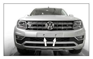
8. Remove the license plate bracket and unscrew 2 bumper mount screws.
