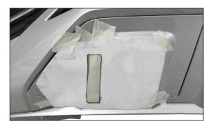
52. Place the template to the bumper. Align the faces marked on the template with the bumper faces and fix them with scotch tape. Pre-paste over part of the bumper at place of cutout with painter's tape for easier marking.
