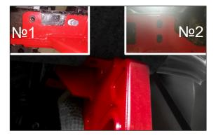
24. Place the left recovery point to the vehicle frame from outside; match the holes number 1 and number 2.
