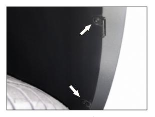
4. In the wheel arches of the vehicle unscrew 2 screws securing underwing flap to the bumper on each side.
