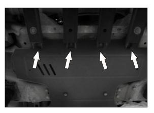
23. If towing hinges are installed the OE skid plate, first install the skid plate, using the rear mounting points (see step 14).
