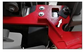
42. Install the bolt M16x120 with washers pos. K, and the nut M16 on the inside of the frame as shown.
