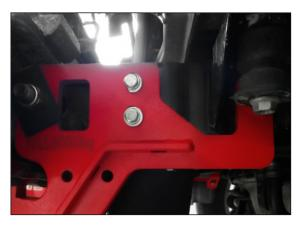
33. Install the washer pos. K, and nut M16 on the bolt M16, on the side of the recovery point.
