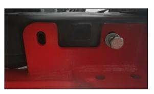
27. Place the left recovery point (see step 21) to the vehicle frame, tighten the bolts M8x40 in the holes number 1 at the bottom of the recovery point.
