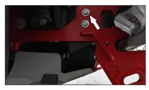
40. Place the recovery point and screw 2 bolts M8x40.
